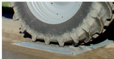
The drive-over-scale also weighs large low pressure tyres.
