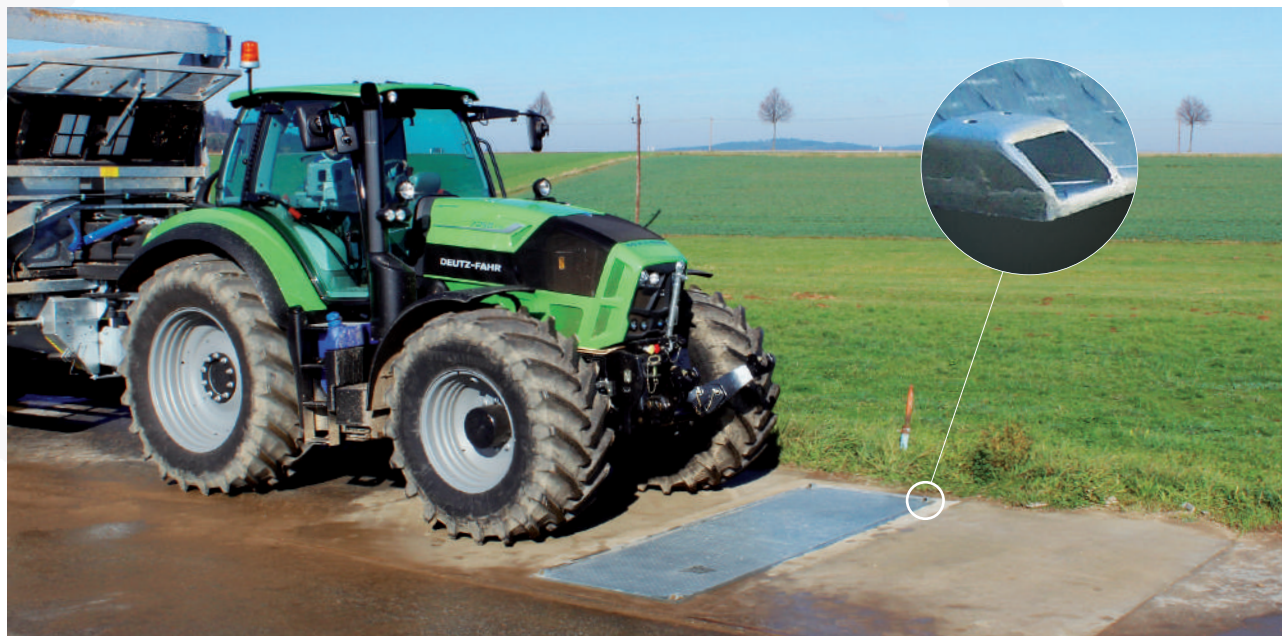
Axle recognition through light barriers.
